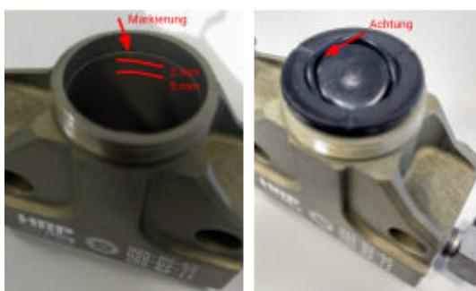
The compensating membrane must lie cleanly and must not be "bent". After use in the rain, absorb any moisture between the cover and the compensation membrane with a cloth.
